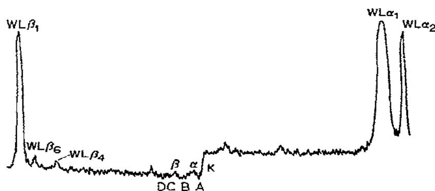
Fig. 10. Microphotometer record of K -absorption edge of copper in Cu-TPA complex.
